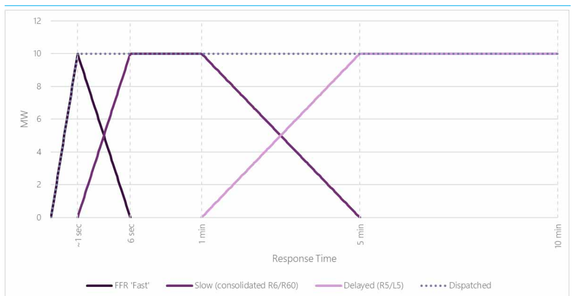
Figure 3.3: Option 2b: Reconfiguration of the contingency raise services to include FFR – consolidation of R6/L6 and R60/L60
