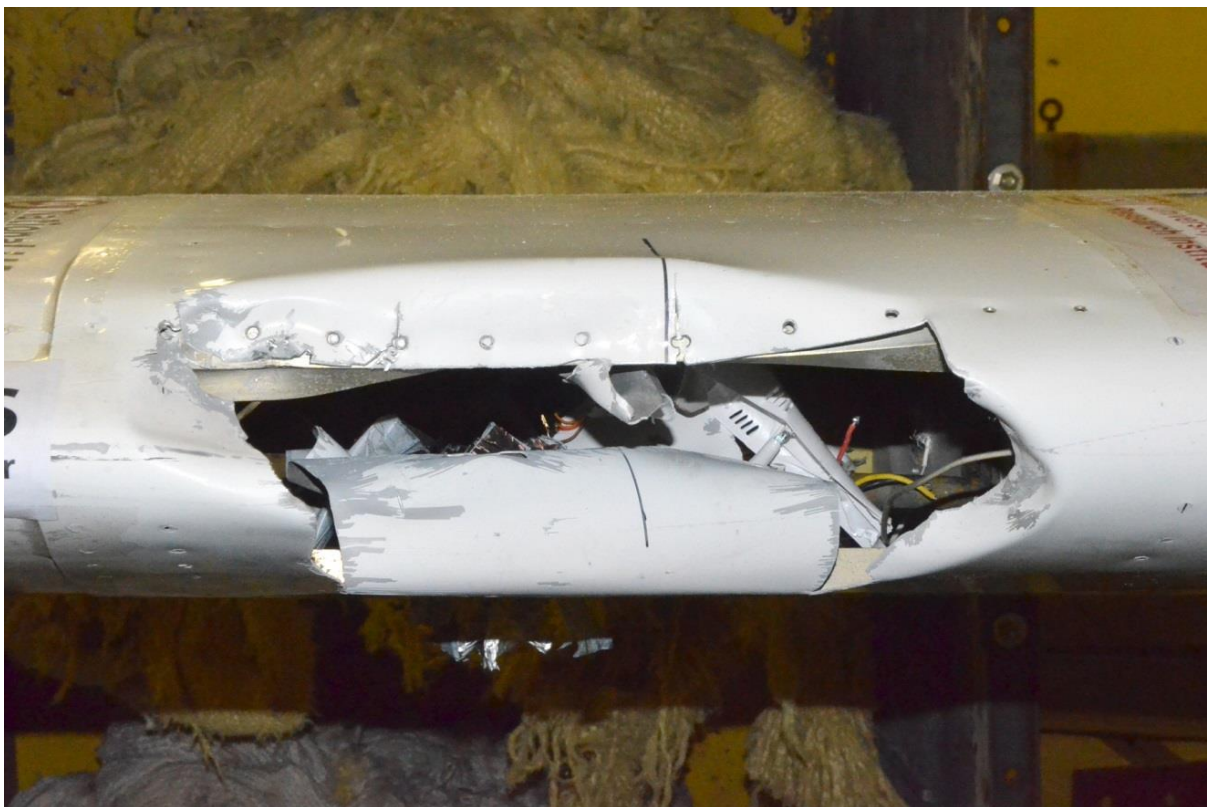
Image 1. Damage to the leading edge of a Mooney aircraft by a simulated 1kg RPA impact. Source: University of Daytona Research Institute
