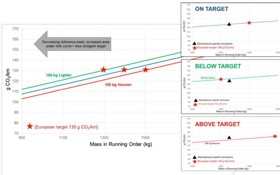
Figure A2: Effects of a change in average vehicle mass under the EU standards (ABMARC 2016)
