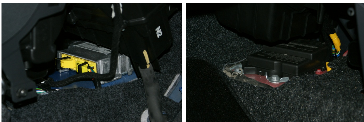
Figure 14 North American market vehicle (left) and Australian market vehicle (right) airbag control modules (Model A)
