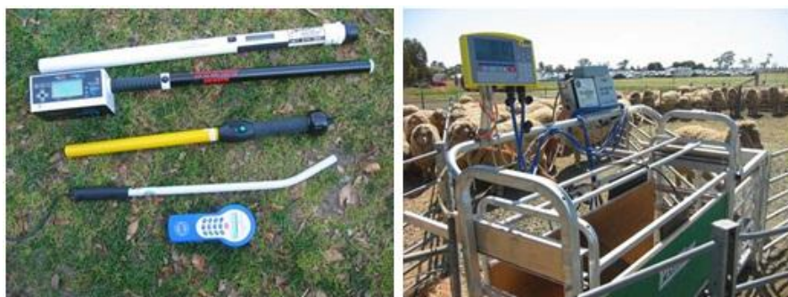
Figure 7 Electronic scanners—handheld scanners and panel reader
