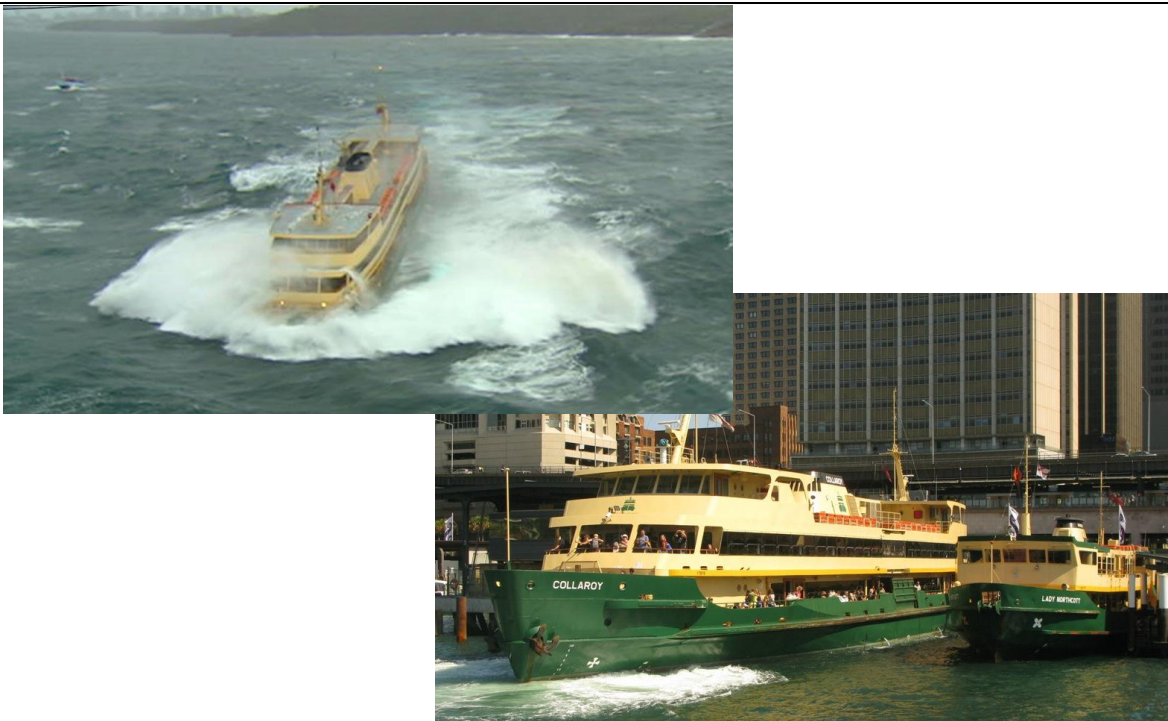
Figure 4 — (Top) Manly ferry in extreme partially smooth water conditions – Photo: ABC TV. (Bottom) Manly ferry showing arrangements for additional bow height – Photo: Mori Flapan
