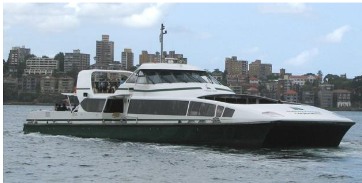
Figure 5 — Ferry design found to have insufficient bow height for Manly service – Mori Flapan
